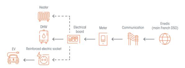
For buildings not equipped with HEMS, the Linky meter is capable of transmitting signals to the electricity supplier's grid (index, no prices in  $\pounds$ ).
