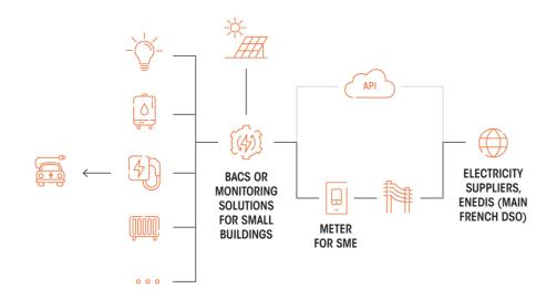
Theoretically, controlling the DSO Commercial & Industrial Metering through the ICT provides real-time access (instantaneous power extracted and maximum power limit, ongoing pricing period, start and end date of mobile Peak times) which can be interpreted by the BACS.
