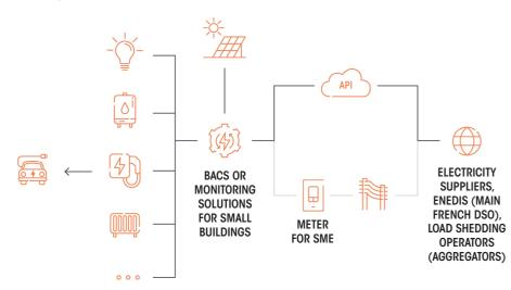
Request via ICT and metering chain through BACS (>70kVa and >36kVa)
